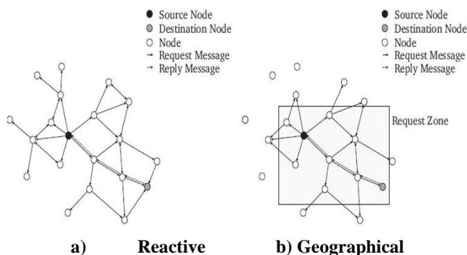
**Figure 3: MANET Routing Algorithm**
